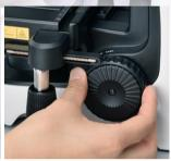
Coarse/fine focus and stage movement can be operated with one hand
