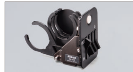
Shutter cassette for Ni-L (Ni-L) By blocking light from the LED light source and autofluorescence, this unit allows acquisition of high S/N fluorescence images without the need to turn off the diascopic illumination.
