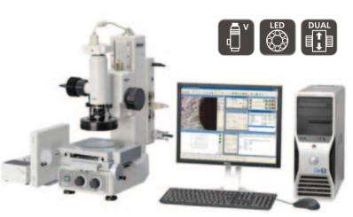
MM-200 with C-mount Video Head and E-MAX DS-V
