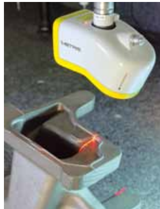
Scanning of casting
