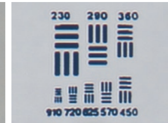
Resolution chart (Objective: TU Plan Fluor 10x)
