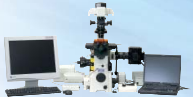
Configuration with Nikon C1 confocal imaging system, Epi-FI and TIRF imaging systems
