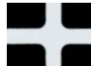
The target in the viewfinder allows easy manual focusing.
