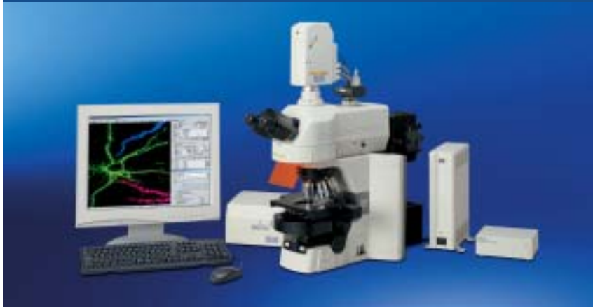
ECLIPSE 90i configured with the digital-imaging head DIH-E, confocal microscopy system C1, and digital camera DS-5Mc-U1.
