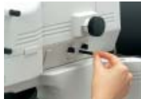
Adjustments can be made by simply sliding the excitation balancer back and forth.
